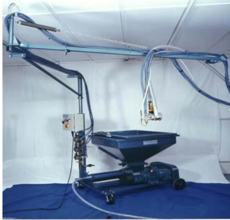
Photo H.C.3 fitted with M/C Boom and P111 Concentric Gun
